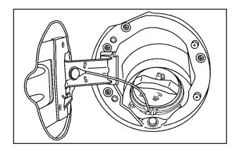
The tethered fuel cap is located behind a hinged fuel door on the driver side of the vehicle.
